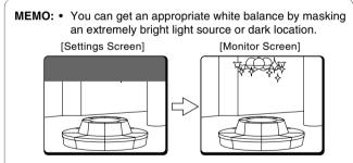
While setting the area, the masking is shown but is not visible on the monitor screen.
